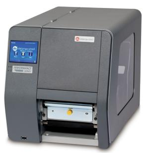
The Performance Series printers are available with numerous options to meet the most diverse requirements. Some of the options include internal rewinder, peeler and cutter, USB host, GPIO, 802.11 b/g and audio alarm.
