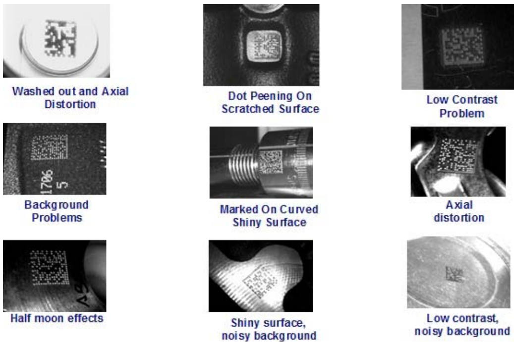
Figure 7 - Problematic Direct Part Marking Examples
